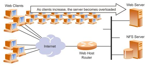
Figure 6-2 Web Hosting Configuration Without SLB
